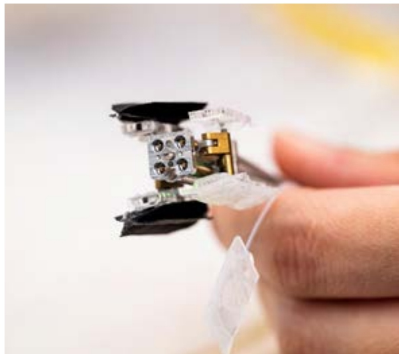
MIRACLE from the University of Basel: A robotic endoscope for precise, minimally invasive bone and cartilage surgery.
