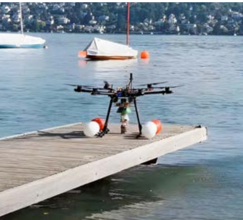
Helping fight the quagga mussel: The Medusa air-water vehicle developed by EMPA Dübendorf.
